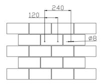
Figure 4.6 Drill holes' dimensions of R5-3K/4K/5K/6K/8K/9K/10K/12K-T2 R5-3K/4K/5K/6K/8K/9K/10K/12K-T2-15
