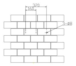
Figure 4.8 Drill holes' dimensions of R5-17K/20K-T2
