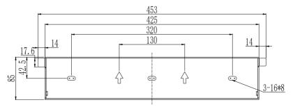
Figure 4.5 Dimensions of rear panel of R5-17K/20K-T2
