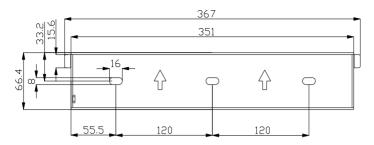
Figure 4.3 Dimensions of rear panel of R5-3K/4K/5K/6K/8K/9K/10K/12K-T2 R5-3K/4K/5K/6K/8K/9K/10K/12K-T2-15
