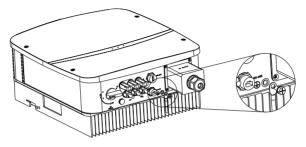
Figure 5.9 Inverter ground protection
