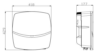
Figure 3.2 Dimensions of R5-3K/4K/5K/6K/8K/9K/10K/12K-T2 R5-3K/4K/5K/6K/8K/9K/10K/12K-T2-15
