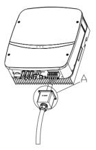
Figure 5.10 Connecting the cable
