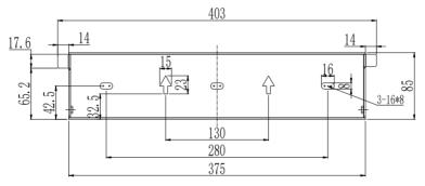
Figure 4.4 Dimensions of rear panel of R5-13K/15K-T2
