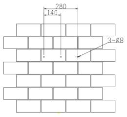
Figure 4.7 Drill holes' dimensions of R5-13K/15K-T2
