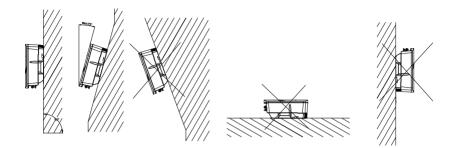
Figure 4.1 Mounting method
